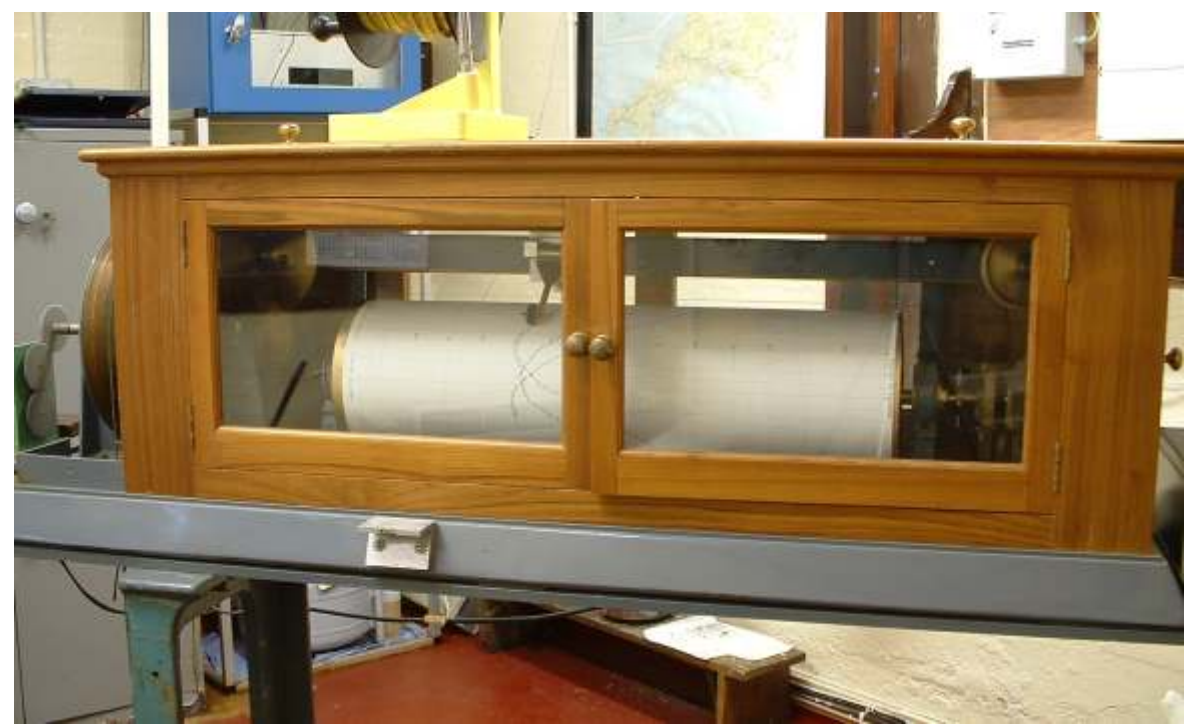
Newlyn chart gauge. The charts come from tide gauges around the UK and have been digitised as 15 minute interval data.
